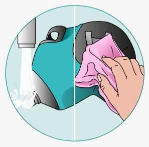
**13** Clean the exterior of the IDAL. Only the head and the spike can go under the tap.
